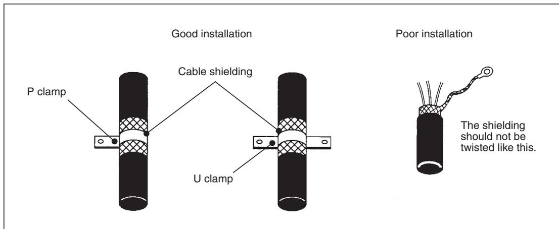
Route control signal cables at least 30cm away from all power cables. Do not route the power supply cables or the cables connecting the frequency inverter and the motor in parallel to control signal cables, telephone cables or data cables.
