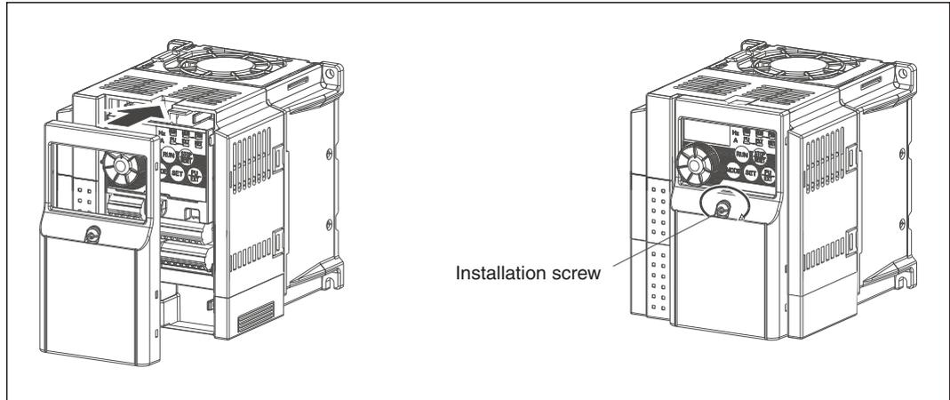
**Removing and replacing on models FR-D740-120 and FR-D740-160**
