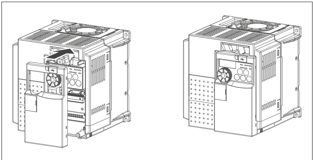
**Removing and replacing on models FR-E740-230 and FR-E740-300**
