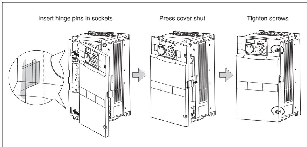
**Removing and replacing on models from FR-F740-00770/FR-A740-00770**
