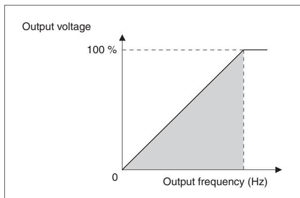
The speed of the connected motor can be adjusted continuously by changing the output voltage and frequency of the inverter.
