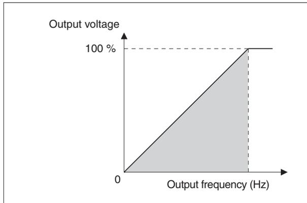
Parameter 3 defines the ratio between the output voltage and the output frequency (V/f pattern).
