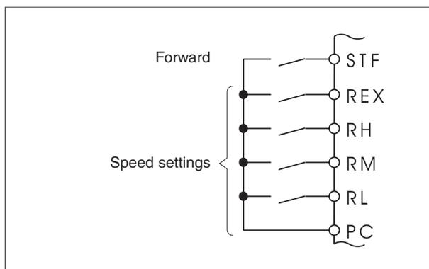
Example for connection of the inverter's RH, RM, RL and REX terminals.
