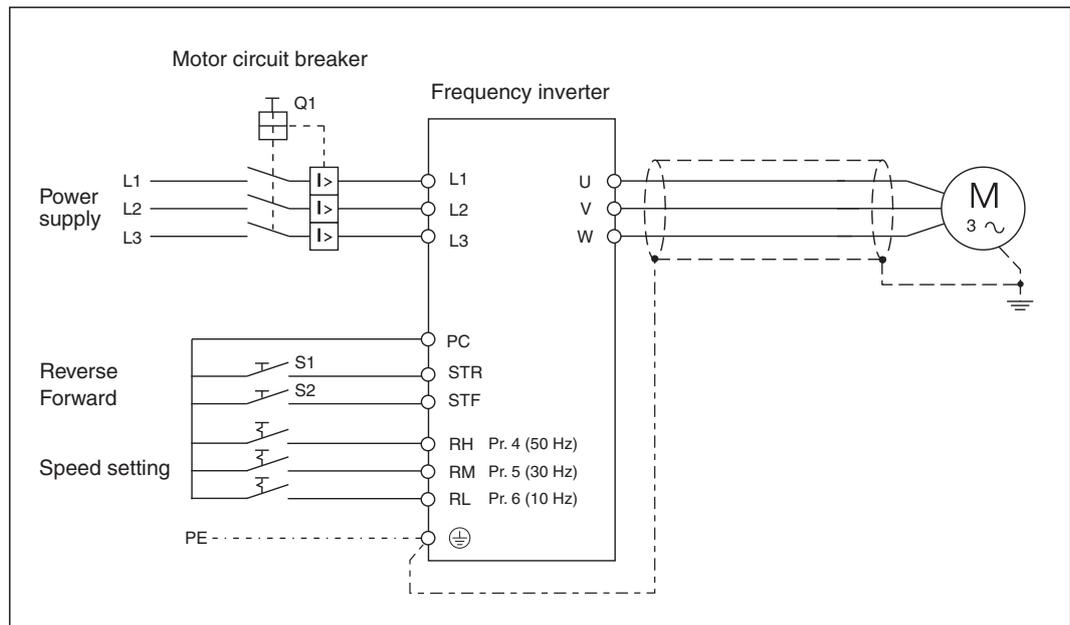
Some external components like pushbuttons and switches are required for this method but it has advantages over performing the test with the integrated or external control unit:
