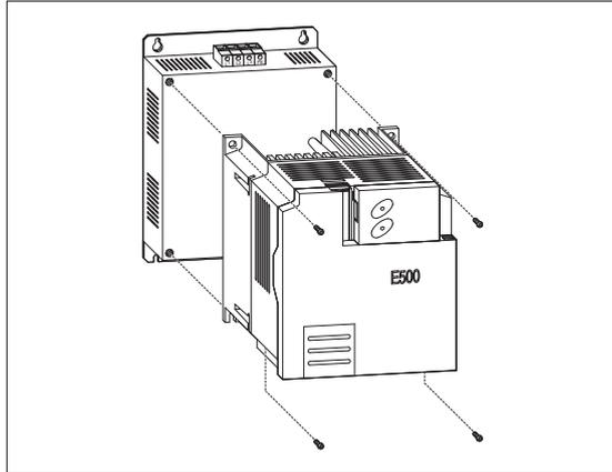
The EMC filters of the FR-D700 and FR-E700/E700S series are installed beside or behind the inverter, depending on their design. Installing the filter behind the inverter has the advantage that the filter does not take up any additional space in the switchgear cabinet.
