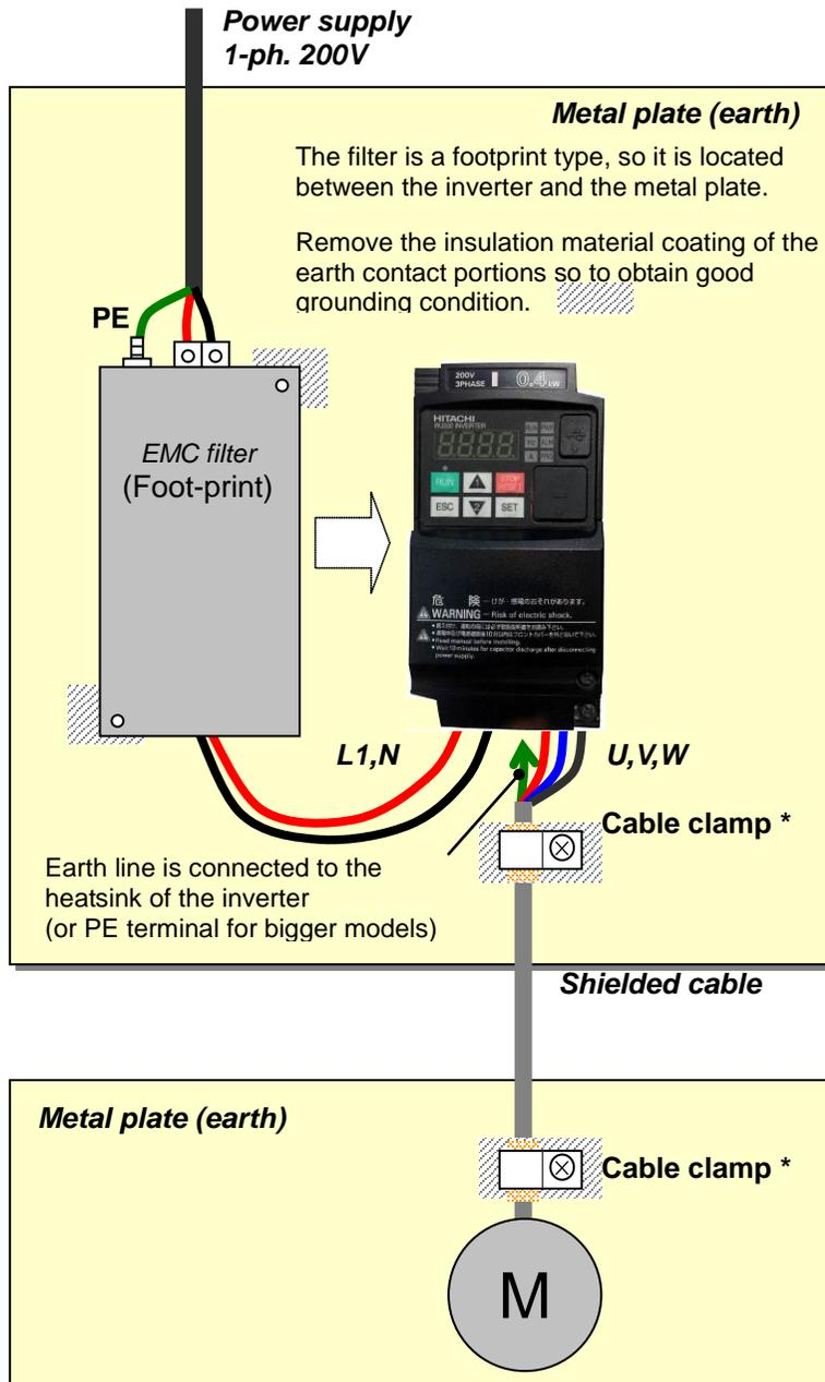
\*) Both earth portions of the shielded cable must be connected to the earth point by cable clamps.
