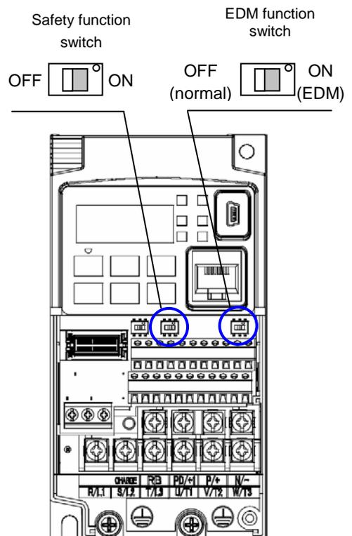
please turn the EDM function switch on. EDM output is automatically assigned on intelligent output terminal 11.
