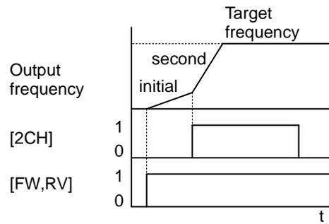
In the graph shown above, the [2CH] becomes active during the initial acceleration. This causes the inverter to switch from using acceleration 1 ( $\Phi 002$ ) to acceleration 2 (**A092**).
