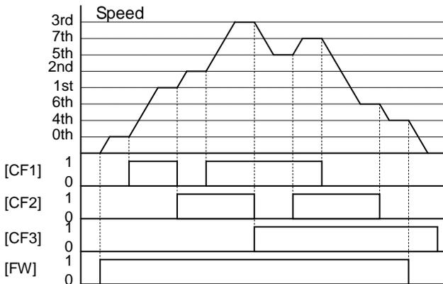
The example with eight speeds in the figure below shows how input switches configured for CF1–CF4 functions can change the motor speed in real time.
