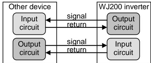
In order to avoid equipment damage and get your application running smoothly, we recommend drawing a schematic of each connection between the inverter and the other device. Include the internal components of each device in the schematic, so that it makes a complete circuit loop.
