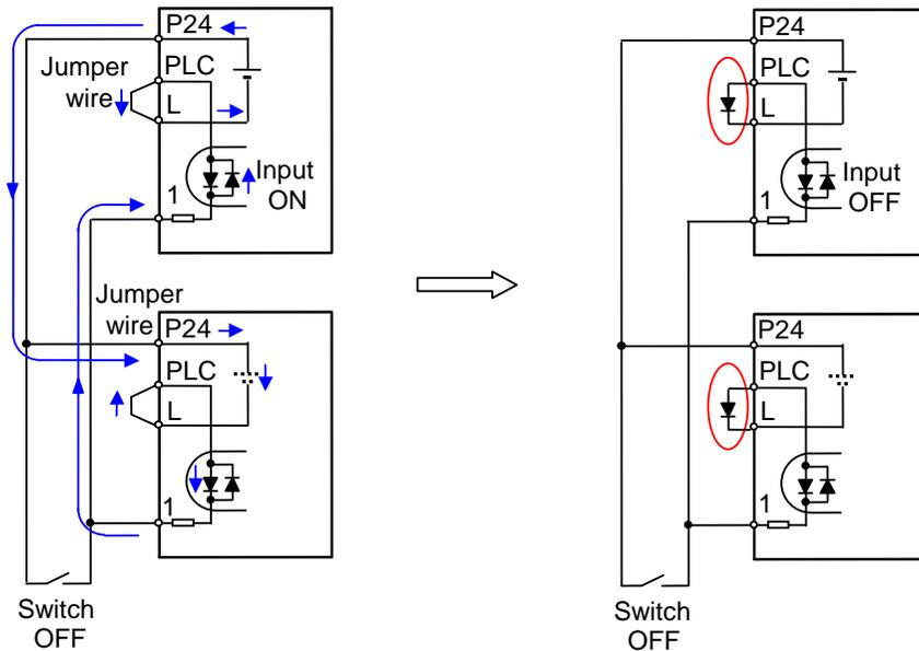
The current loop cause turn the input ON even the switch is off when diode is not inserted.
